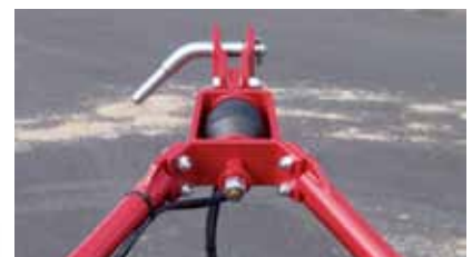
Rubber buffer for protection of machine and tractor.
