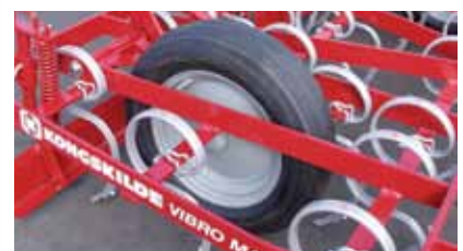
Wheel 165 x 15" standard for SQ. Wheel 6.00 x 12" standard for SGC.
