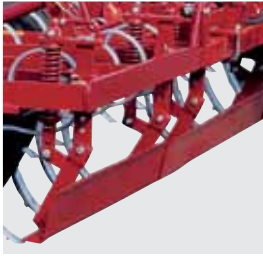
SPAGC levelling bar For all types of soil. Levels and crumbles the soil in front of the machine.
