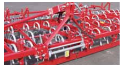
Semi-quick hitch for easy coupling.
