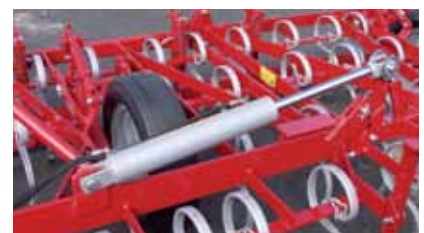
Folding and unfolding with double-acting cylinders.
