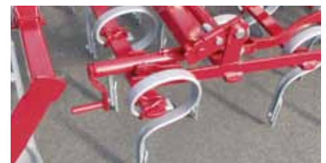
The working depth is adjustable by the means of a spindle on each section.
