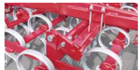
By releasing the four catches on each tine section, the section can be removed from underneath the Germinator when changing the shares.
