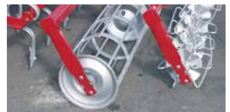
The cage rollers support the machine in its working position.
