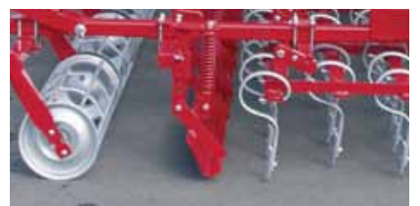
Spring loaded adjustable levelling bar.
