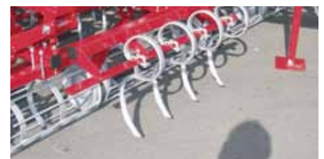
Track eradicator kit for all models is available as an optional extra.
