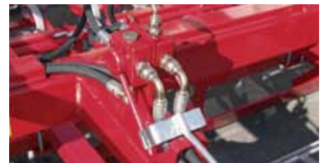
The Germinator is equipped with 3 hydraulic systems but only a double acting hydraulic system is required on the tractor.
