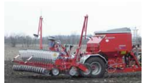
Aeromat C "E-motion" 16 DTE in conjunction with trailed fertiliser hopper Aeromat "Maxi-Line".
