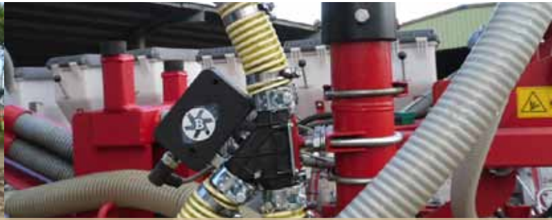
Magnetic flap valves for fertiliser distribution 16 / 8 rows (optional).
