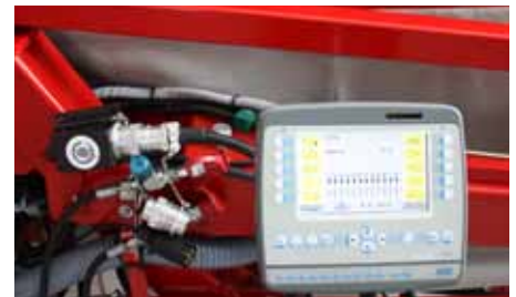
ISOBUS connection and the standard Field-Operator 300 terminal.
