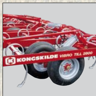
The walking tandem wheels ensure an even working depth in uneven conditions.
