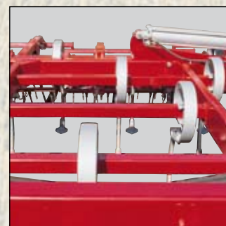
The tines are mounted on sturdy square profiles.
