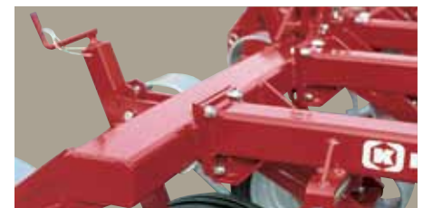
VF 4200 / 4300 / 4000 Rubber wheel 24 x 8.00 - 14.5 with spindle adjustment.
