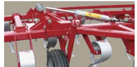
VF 4200 / 4300 / 4000 Folding with double acting cylinders.
