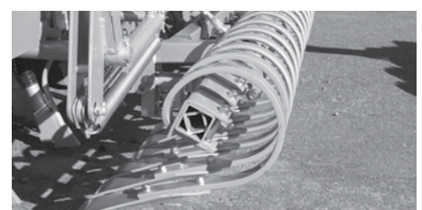
The levelling board creates the final seedbed before drilling.
