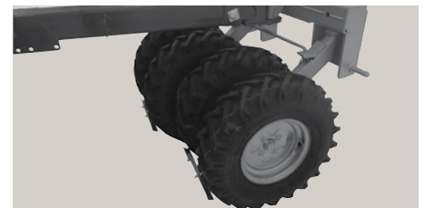
The HT models can be equipped with an interwheel packer to reconsolidate the area between the tractorwheels.
