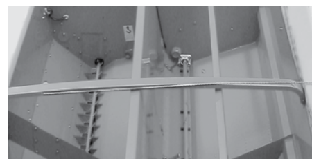
HT 3000 S and HT 4000 S have movable middle wall and agitator in both hoppers.
