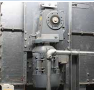
Compact drive solution with bevel gear motor.
