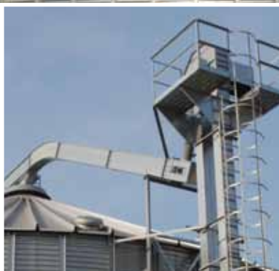
KCA chain conveyor with angle section from inclined to horizontal conveying.
