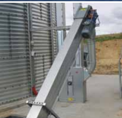
Chain elevator for filling silos.
