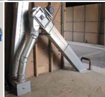
Chain elevator from the grain pit delivers the grain to the flexible foot on the next elevator.
