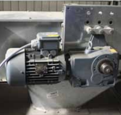
Bevel gear motor with high efficiency.
