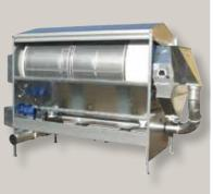
Screen drum with 2 layers of screens. The Inner screen works as scalping screen retaining oversize impurities. The outer screen is a sand screen where small impurities are sorted from the prime product.
