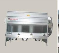
KDC 4000 model with outlet hoppers, without auger. Ideal for cleaning crops with large impurities such as maize.
