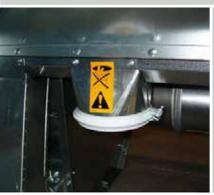
The first bottom outlet can be opened, if you want to collect small kernels together with the screenings from the outer screen.
