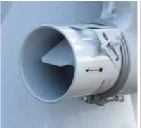
Air regulation for adjusting the suction power of the aspirator.
