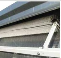
Cleaning brush ensures optimum cleaning af all times by keeping the outer screen clean.
