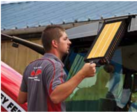
● The cab air filter can be removed easily for cleaning
