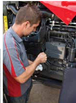
● The waisted bonnet and front axle design ensures comfortable access to the engine oil filters and oil dipstick
