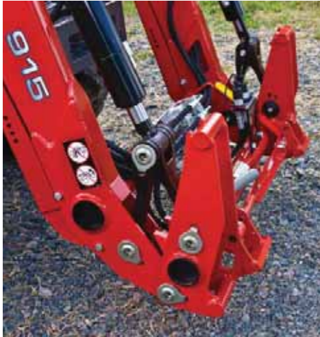
The tool carrier This provides a secure link between the loader and implement, ensuring safety and security during all loader operations.
