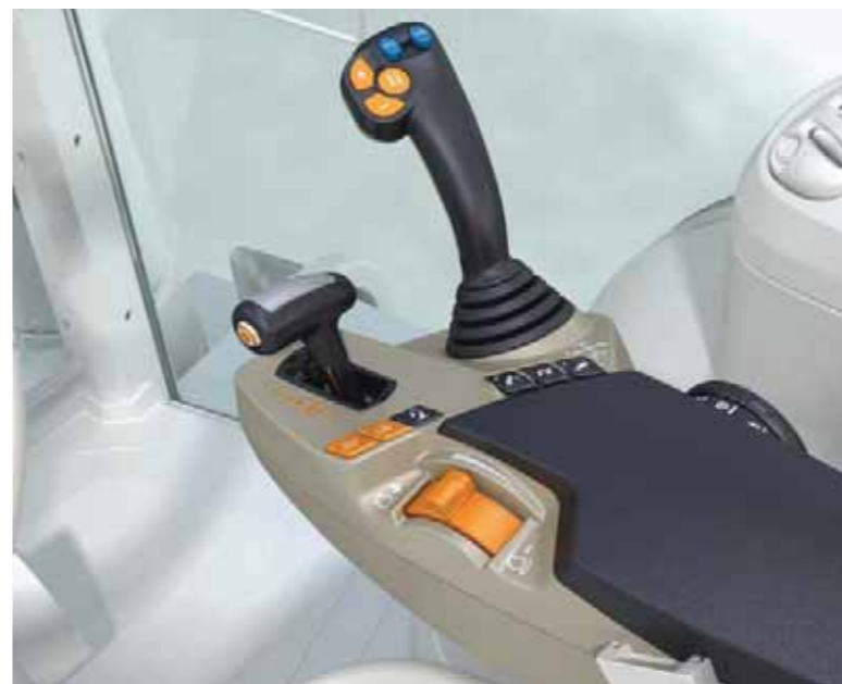
MF 7600 Series Efficient cab option with electrohydraulic multifunction joystick and armrest
