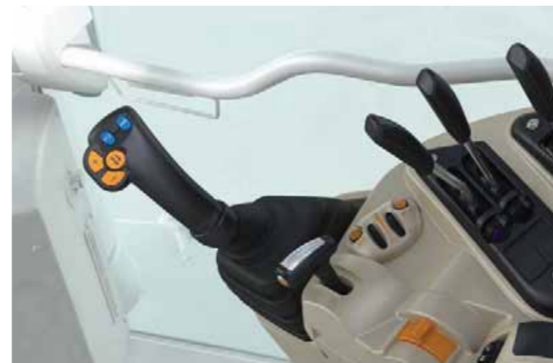
MF 7600 Series Essential cab option with mechanical multifunction joystick
