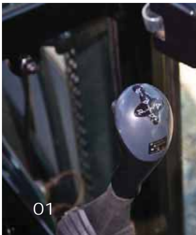
01. The mechanical joystick functions: • Lift • Lower • Crowd • Dump
