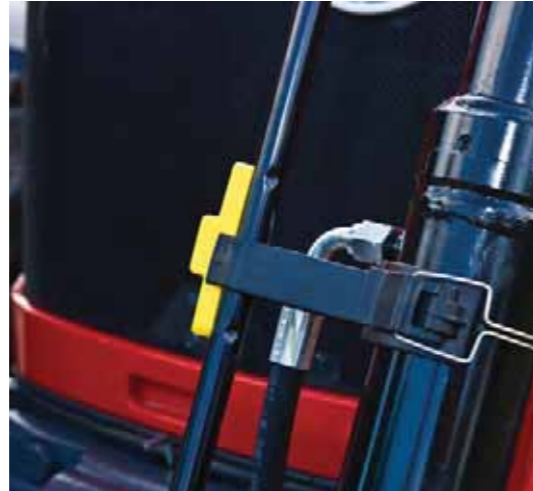
Adjustable guide The guide indicates to the operator the position of the implement. It is easily adjustable and, for example, can show when the bucket or pallet forks are parallel to the ground.
