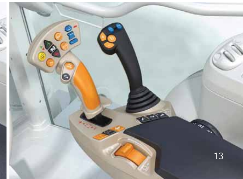
MF 7600 Series Exclusive cab option with multipad control lever and electrohydraulic multifunction joystick (right-hand side)
