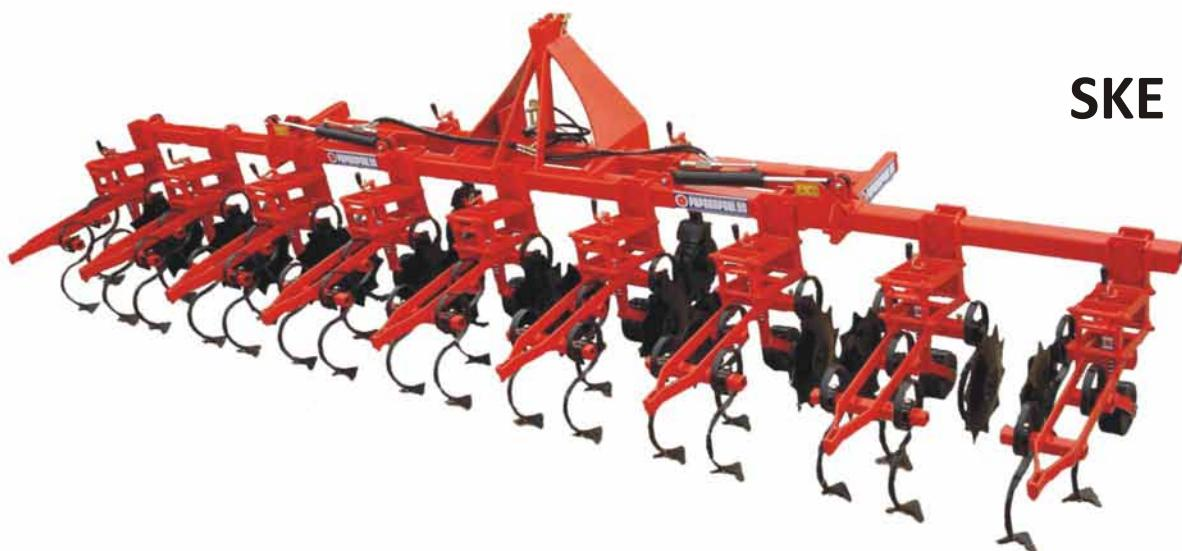
The main frame, on all models of SKE and SKLE series, is made of a robust 3 point hitch and of a double row square tube frame. The frame, of the hydraulically foldable versions, is distinguished from the low wear and a few service points. The ground clearance is kept constant thanks to the infinitely adjustable Jockey wheels which support the main frame. That ground clearance which can be up to 80cm is allowing the processing of even developed crops.
