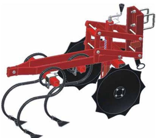
The tool gangs are attached to the main frame by parallel linkage assemblies that consistently keep each sweep moving independently at its desired depth in uneven terrain and independently of any fluctuations of the tractor. A gauge jockey wheel on each tool gang is responsible for accurate depth control.
